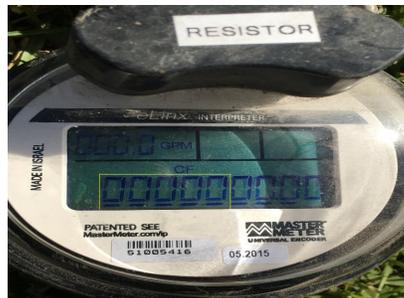
The 5 dials left to right appear on the water bill. The 5th dial is the first billing unit or BU. The rate of flow when water is measuring on the meter can be seen in the upper left and is measured in gallons per minute. The leak indicator is in the upper center of the register and will show an arrow with a (+) symbol for positive registration or an arrow with a (-) symbol for negative registration.
