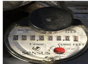
The 4 dials left to right appear on the water bill. The fourth dial is the first billing unit. The red dial is the leak indicator.
