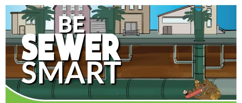
Overflowing sewers are often caused by blockages from FOG (Fats, Oils, and Grease), which can damage homes and businesses. Don't be a pain in the drain. Always scrape, wipe, and toss FOG into the trash.
