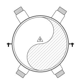
STAINLESS STEEL BAND SPACER & INSULATOR (CONFIGURATION WILL VARY)
