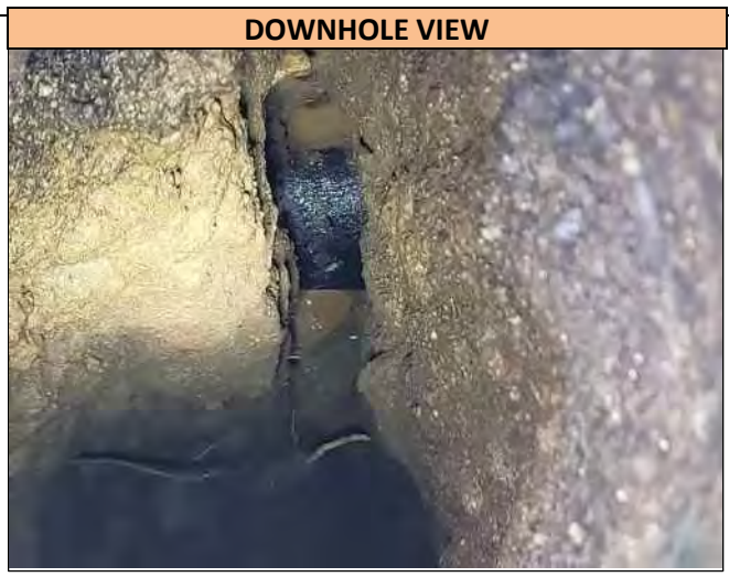
A downhole view of the 6.0 inch wide Steel Water utility found in Pothole 4, at the depth of 55.0 inches T/P. Utility runs in a N/S direction at the Pothole location and was found directly on markout.
